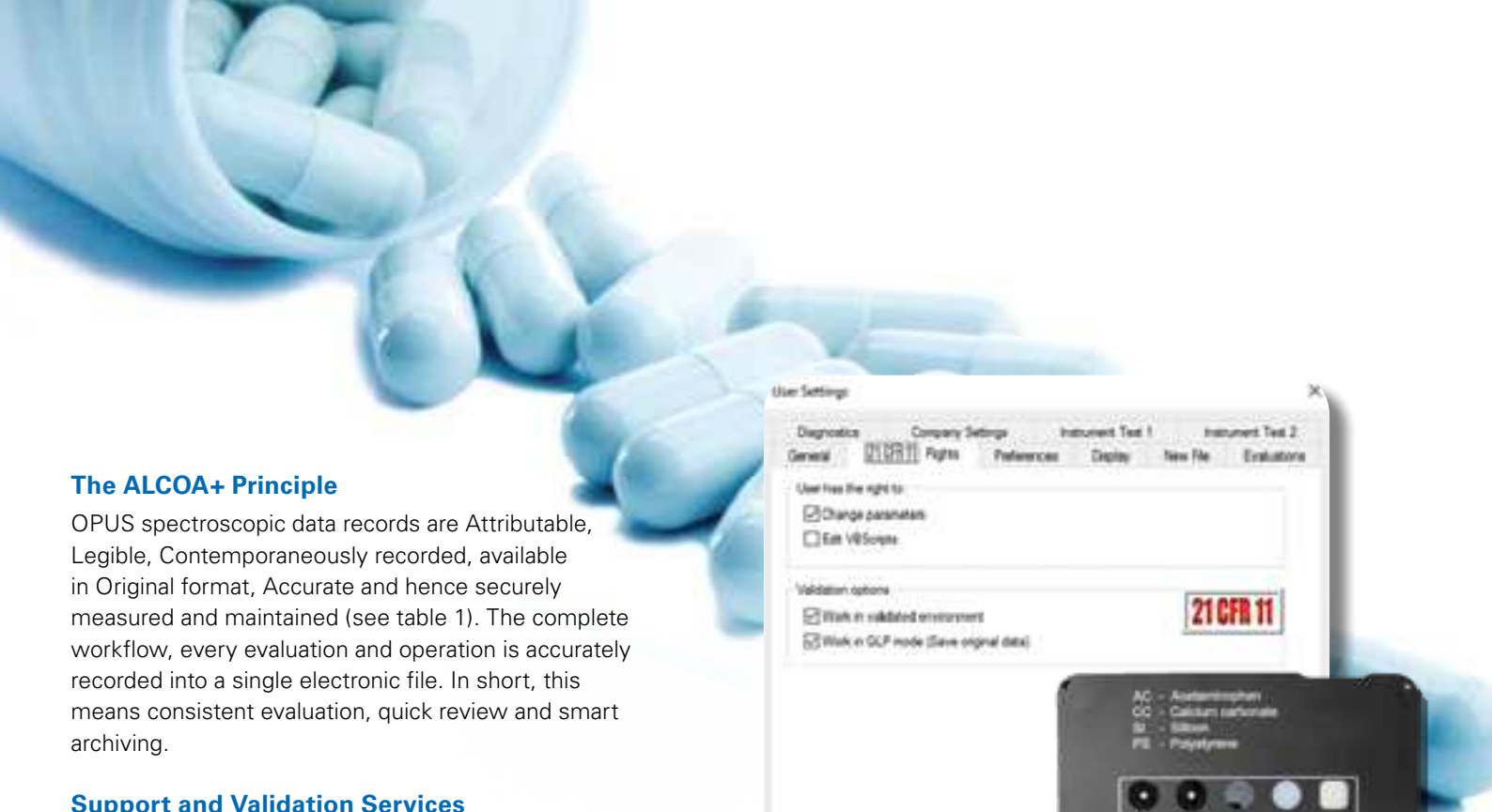
Figure 1: Screenshot of the activated data integrity mode (top) and the SENTERRA II validation plate (right) for automated instrument qualification.
